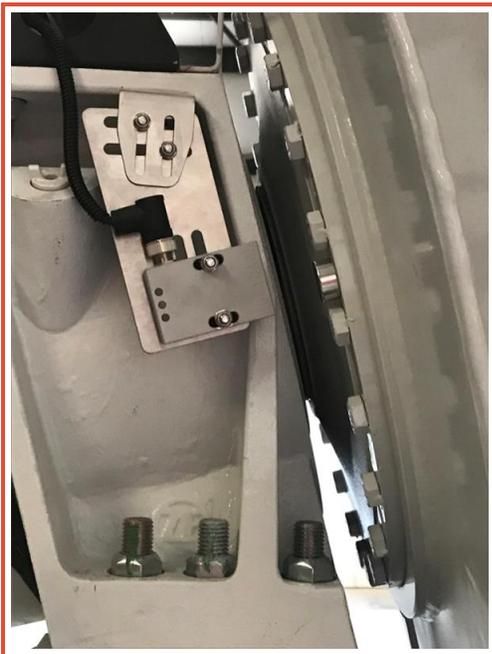
Typically, four (4) magnets are installed with even spacing around the flange. These are often done between existing bolts on the flat flange surface as shown above.
