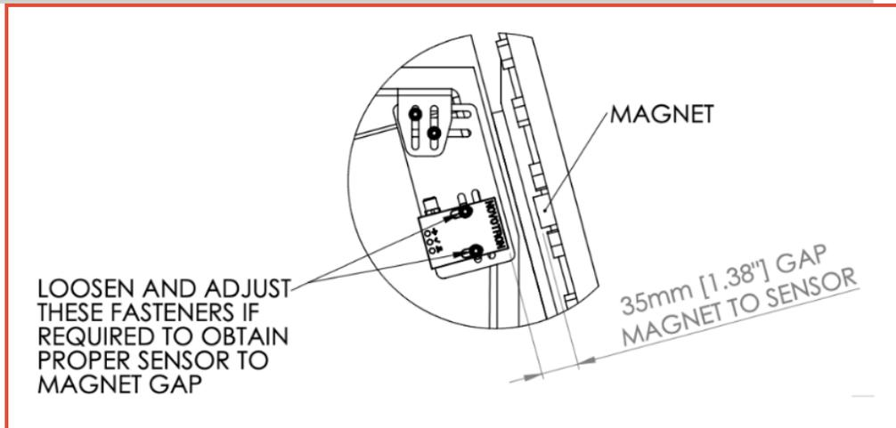
4. Slide the upper bracket in or out to position the center of the magnetic sensor in line with the magnet path.
